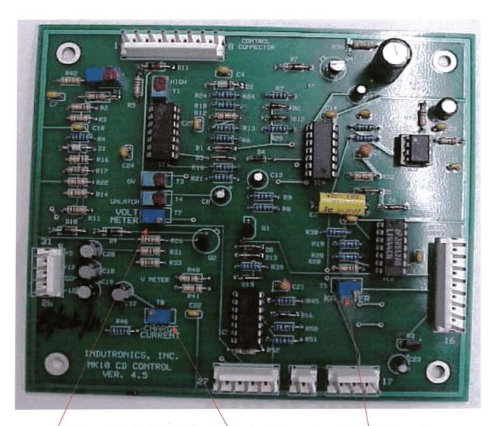
Adjust Volt Meter Adjust charging Current Adjust Current Meter
